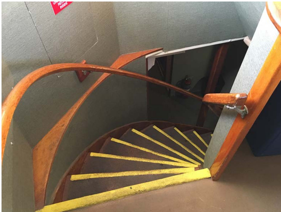
Figure 10. Staircase from the main deck galley/salon leading down to the bunkroom on the Conception . (Source: G. Boyer)
