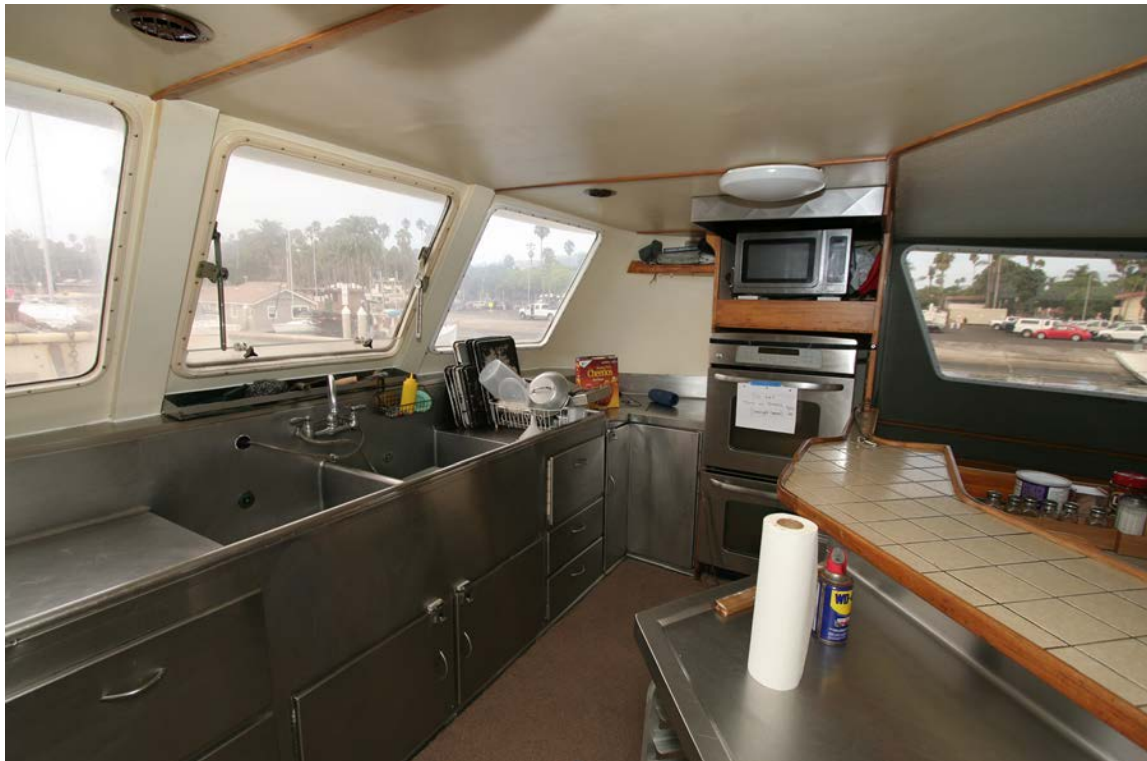
Figure 27. Galley area on the Vision . Note, similar to the Conception , the center window is the only one with hinges that allow for it to be opened.
