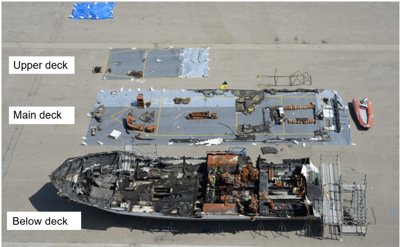
Figure 16. Conception wreckage layout at Port Hueneme. (Source: FBI evidence response team (ERT))
