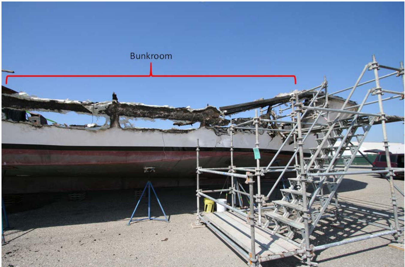
Figure 23. Starboard mid- and forward-section of the Conception hull. (Source: FBI ERT)
