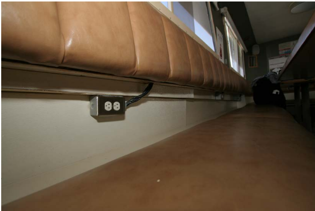
Figure 32. Electrical outlet drop below seatback on the Vision .
