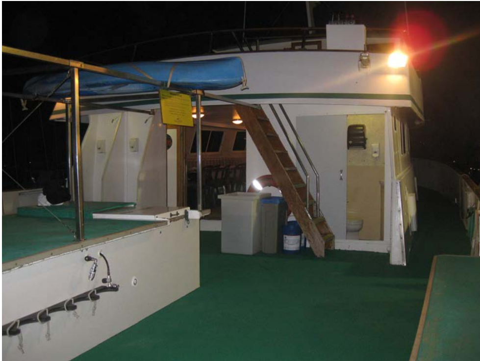
Figure 9. Toilets and stairway to the upper deck of the Conception . Note the storage of a polyethylene trash can, food waste containers, and a rinsing container under the stairway in front of the life ring. (Source: M. Ryan)
