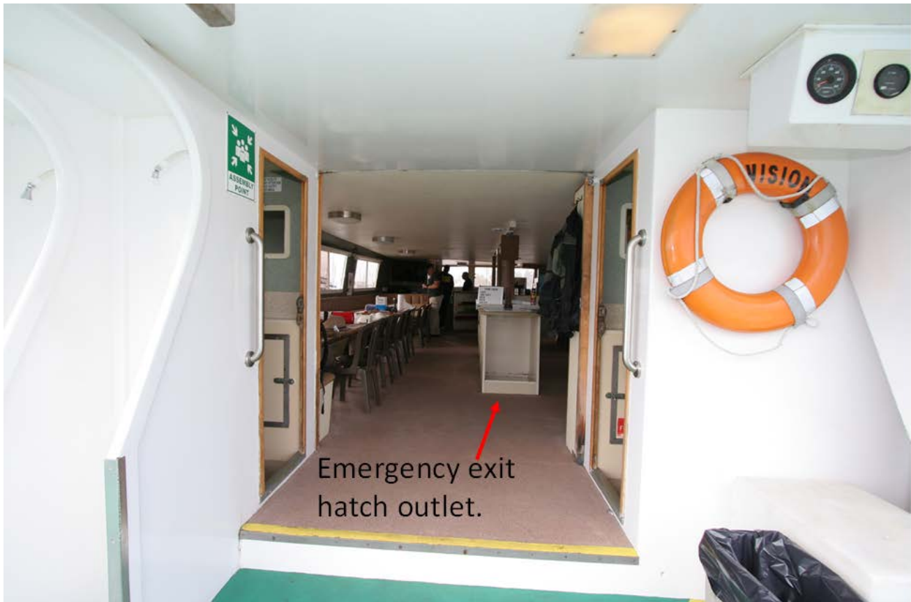
Figure 31. Location of the passenger bunkroom emergency exit hatch outlet in the salon of the Vision .
