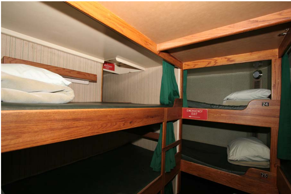
Figure 30. Emergency exit hatch location above passenger bunk on the Vision .
