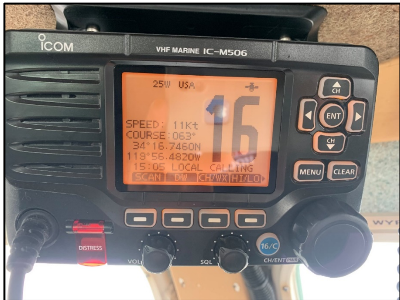
Figure 9: Conception's VHF radio located overhead in the wheelhouse. The VHF-DSC distress button in the lower left is color-coded red. (Source: B. Priddin)
