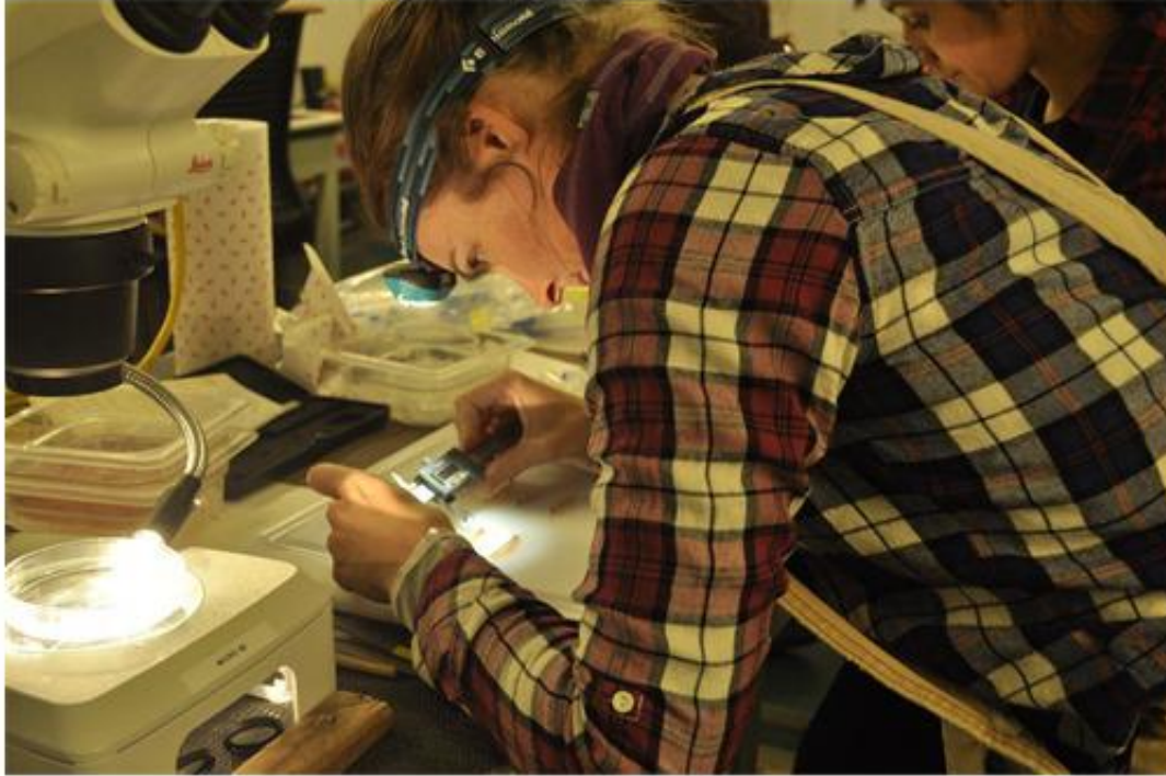
Using calipers to measure krill.
